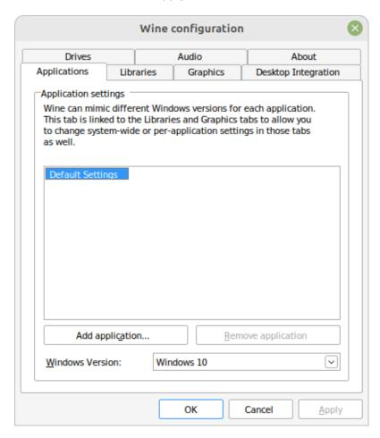
Mouse hovering above the graphs in VituixCAD works properly (as real Windows 10) when 'Allow the window manager to control the windows' in Graphics tab is unchecked, though this disturbs some other functions. Select the setting which suits the best for you.
